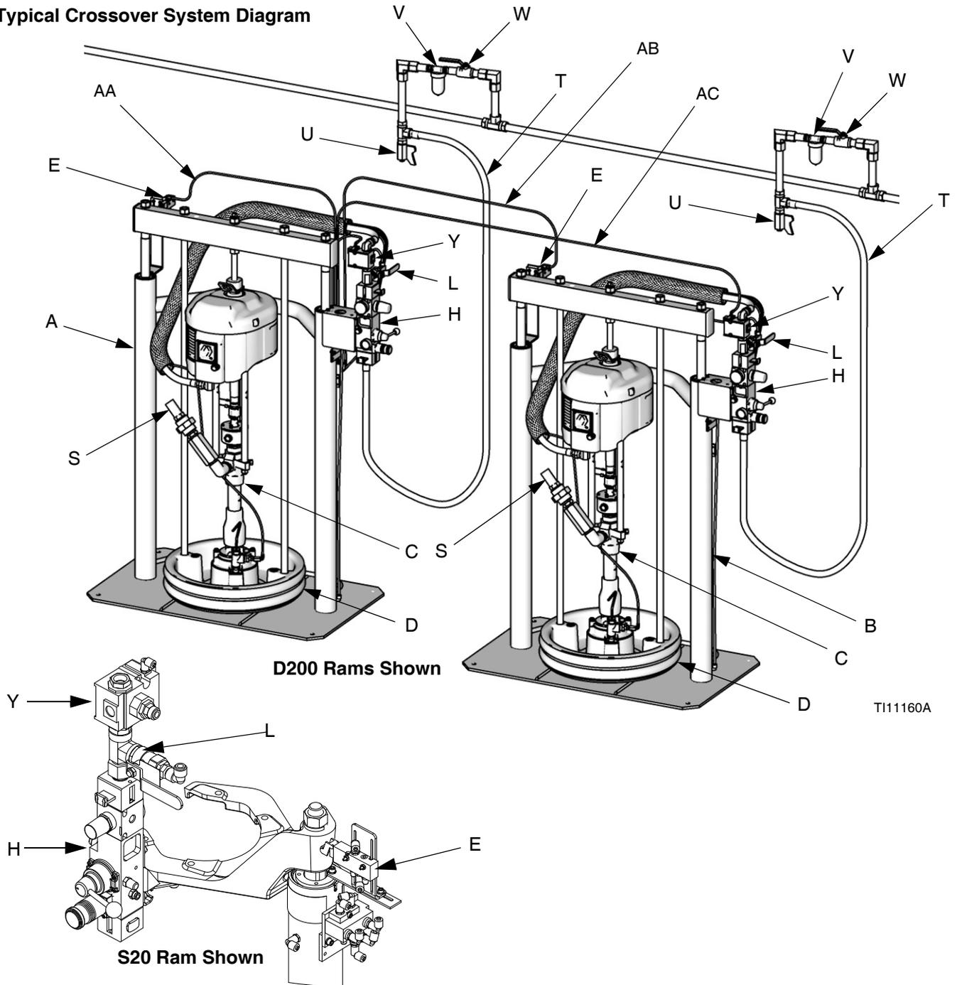
FIG. 1: Component Identification, Pneumatic Crossover
