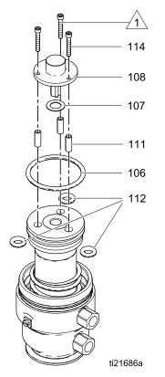
Install assembled air valve from kit: Lubricate and install new o-rings (106 and 115). Use pipe sealant on the threads of the valve (105) and torque to 15 to 20 ft-lb (20.3 to 27.1 N•m). Use a screwdriver as shown, if needed.
