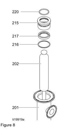
4. Push the displacement rod (202) all the way out the *bottom* of the cylinder.
