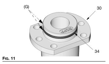
Install the outlet (30) to the spool. Replace and tighten all bolts (37) securely. Torque bolts to 24 to 30 ft. pounds (32.54 to 40.67 N.m) (Fig. 12).
