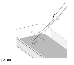
3. Flush the equipment with a compatible solvent until fluid runs clear.
