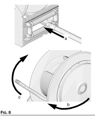
8. Apply pipe thread sealant, or wrap hose threads with PTFE tape.
