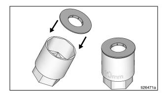
4. Position the push nut and socket at the end of the motor shaft. Use a small or light (8 oz./225g) hammer to drive the push nut onto the shaft compressing the wave washer.
