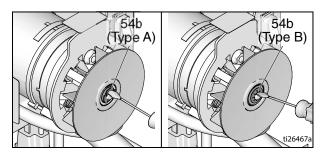
4. Remove and discard old retainer(54b), washer (54c), fan, and shaft adapter (54d). Shaft adapter Type A requires a 5/64" hex key to loosen the setscrew.
