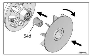
2. Rotate fan clockwise while sliding fan onto shaft adapter (54d) with the fins facing the motor. Slide wave washer (54c) onto motor shaft.
