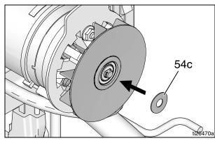
3. Place a push nut (54b) on a 3/8" or 10mm socket.
