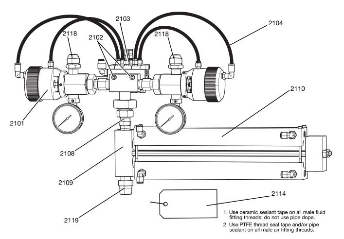
Fig. 22: Tapered Thread Stack 24R681
