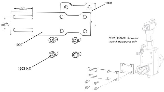
Fig. 20: Stack Bracket Kit
