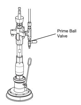
3. To relieve pressure on the side leading out to the stack from the dosing valves, ensure the material outlet valves are open on the A and B side.
