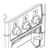
If a second pressure transducer is being used on the F4 System, connect the cable into port 6 for pressure C and port 7 for pressure D on FCM 1 as shown below.
