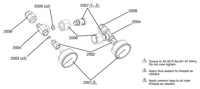
Fig. 21: Stack Adapter Kit
