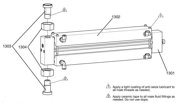
Fig. 14: Straight Thread Two-pass Mixer
