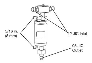
Kit 25A992 has the same components as kit 25A990 and also includes manifold on/off valves and a solenoid block with two solenoids that is designed for systems that are not using a color injector. This kit uses 5/16 in. (8 mm) air line tubing for the air connection between the solenoid block and the manifold valves. There is also a 3/8 in. (10 mm) connection for the stack air inlet.
