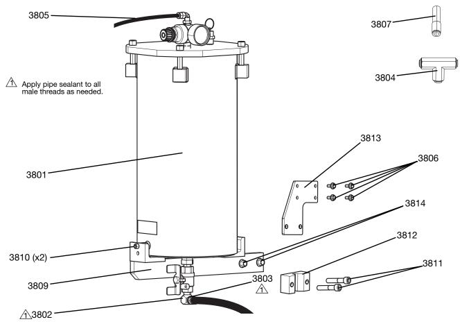
Fig. 39: Colorant Tank 25A105
