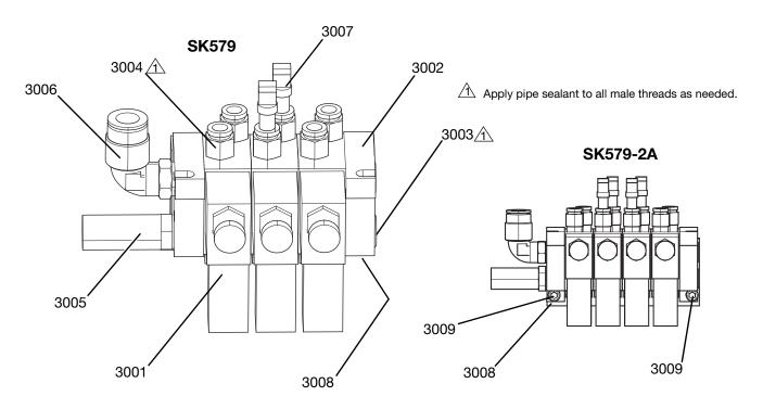
Fig. 31: Tapered Thread Solenoid Block
