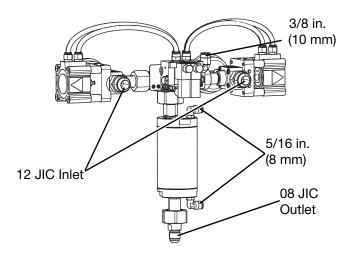
Kit 25A993 has all of the components from kit 25A992 and also includes a color injector (with adapter) and a solenoid block with three solenoids that is designed for use with the color injector. See Color Injector Kits on page 22 for more information.
