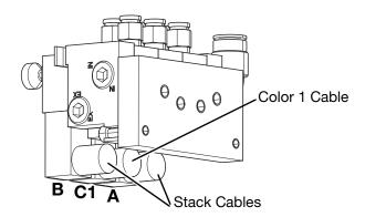
Connect the other end of the cord to the cable included in the kit and connect the cable to the electronic enclosure at the Color 1 connection. See page 9 for a diagram of the electronic enclosure's connections.
