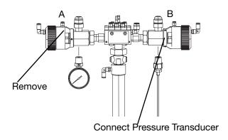
For straight thread stacks, install the 1/2 NPT x 08 JIC adapters (4410) to the stack where the gauges were removed. Then connect the two NPT pressure transducers to the adapters.
