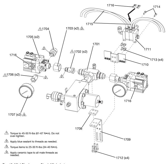
Fig. 18: Mini Single-pass Stack Mini-shots
