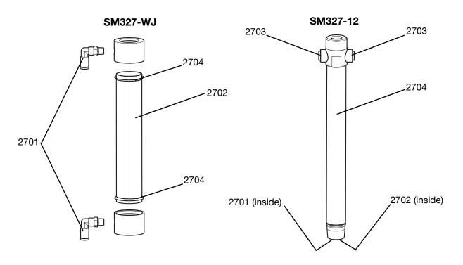
Fig. 28: Tapered Thread Water Jacket and Mixer
