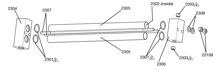
Apply a light coating of lubricant to seals.
