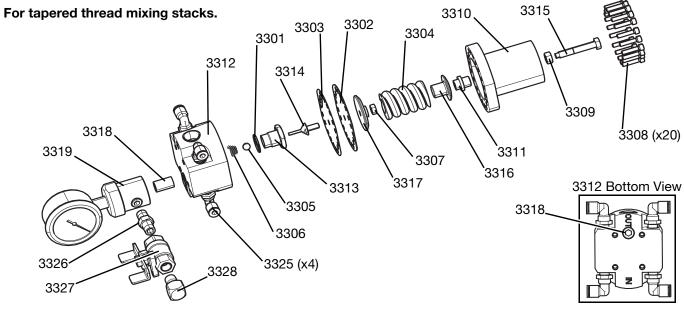
Fig. 34: Tapered Thread Material Regulators
