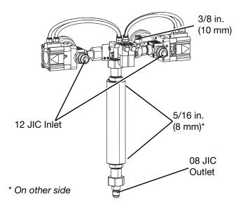
This kit uses 5/16 in. (8 mm) air line tubing for the air connection between the solenoid block and the manifold valves. There is also a 3/8 (10 mm) connection for the stack air inlet.
