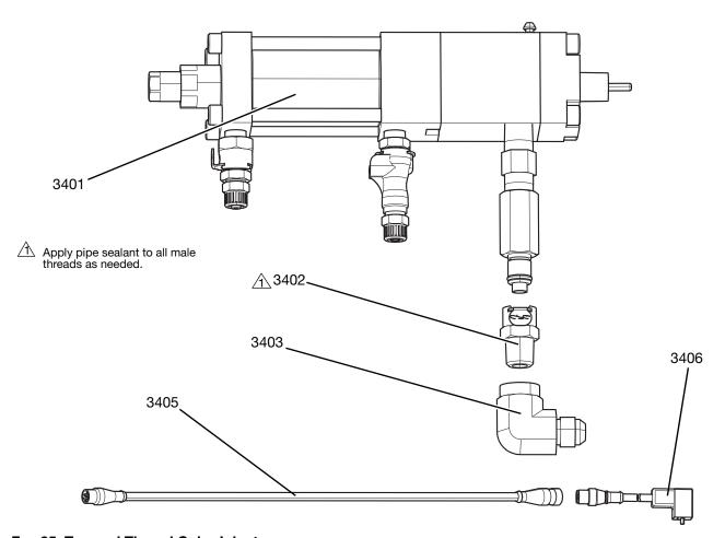
Fig. 35: Tapered Thread Color Injector
