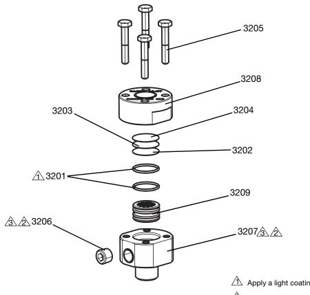
Apply a light coating of lubricant to seals.
