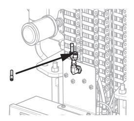
2. Connect the 1/4 in. tubing that is included with the kit to the reducer at the machine.
