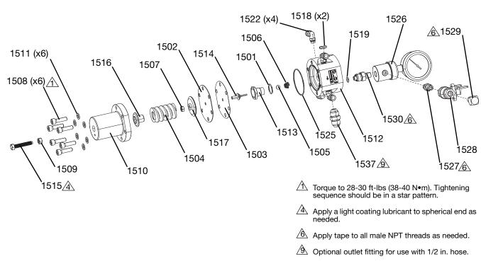
Fig. 16: Straight Thread Material Regulators
