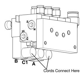
**NOTE:** The number of solenoid block connectors varies depending on which mixing stack you are using.
