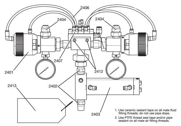
Fig. 25: Tapered Thread Stack 25A169
