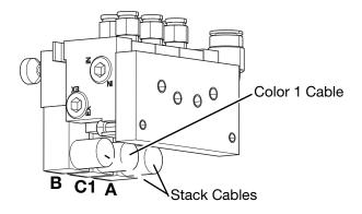
**NOTE:** The solenoid block on mixing stack kit SK556-2A has an extra solenoid for a second color injector (C2). Connect the cable from Color 2 on the electronic enclosure to the C2 connection.
