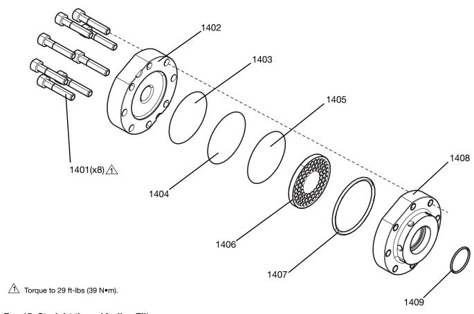
Fig. 15: Straight thread In-line Filter
