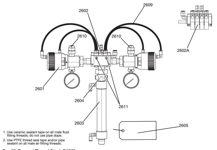
Fig. 27: Tapered Thread Stack SK556
