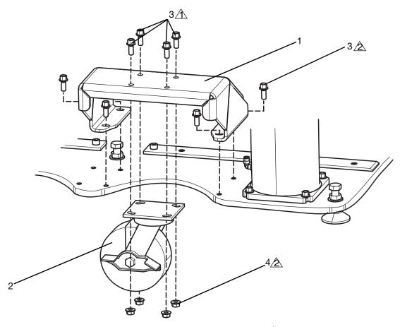
Apply sealant to all male threads as needed.
