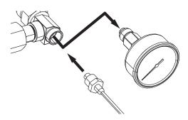
2. Connect each pressure sensor (4403) to the cables (4404) included in the kit and run the cables to the machine's electronic enclosure.
