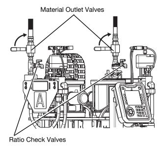
4. Open the ratio check valve on both the A and B side to relieve pressure.
