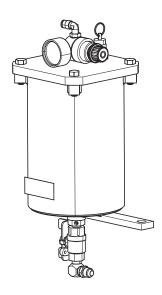
This colorant tank is for use with the F4-5 and holds up to 3 qt (3 liters) of color material. See page 72 in Parts for part identification.
