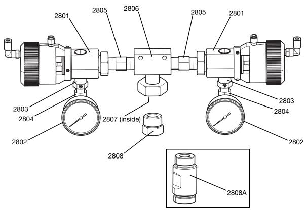
Fig. 29: Tapered Thread Manifold Assembly
