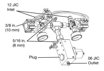
Kit 25C792, which is included as part of kit 25C794, can be purchased and used separately. This kit has the combined mixer-material regulator component with the third valve, but does not include the manifold on/off valves, a solenoid block, or gauges.
