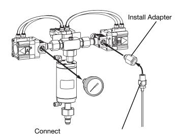
**NOTE:** The pressure transducers can also be used with the stack adapter kit 25D011 (see page **13**). Remove the gauges and install the pressure sensors (4403) directly into where the gauges were removed, as shown below. Do not use the pressure transducer adapters (4405) or the 1/2 NPT x 08 JIC adapters (4410) for this installation.
