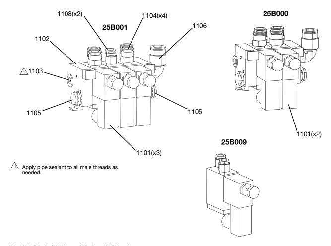
Fig. 12: Straight Thread Solenoid Blocks
