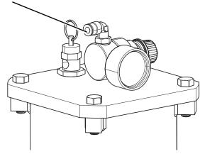
Connect the color material line to the 06 JIC connector at the bottom of the tank.
