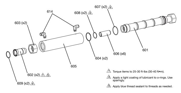
Fig. 7: Straight Thread Single-pass Mixer
