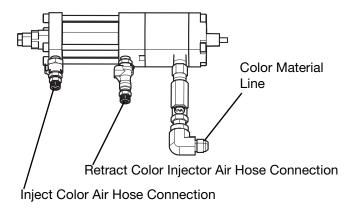
**NOTE:** The disconnect has a check mechanism on both sides to prevent colorant from pouring out when not attached.
