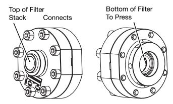
This filter is installed at the end of the mixer, between the mixer and a material regulator.
