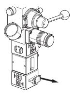
2. Open the prime ball valves for both the A and B pumps.
