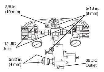
Kit 25C799 has the same components as kit 25C794 except it does not include the third valve for controlling material dispensing.
