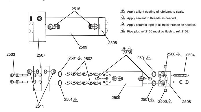
Fig. 26: Tapered Thread Water Jacket and Mixer
