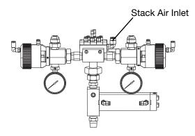
**NOTE:** If two stacks are being used with a dual press setup, use the 3/8 in. air line tee included with the dual press kit (25A102) for the connection at the machine. See **Dual Press Kit, 25A102** on page **7** for information.
