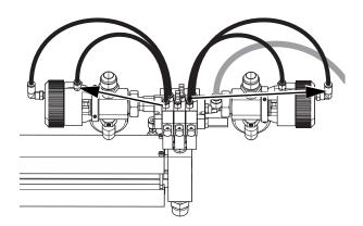
4. After the pumps and material lines have been primed, connect both the A and B material outlet
