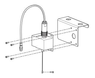
Follow these steps to install the sensors on both the A and B sides.
