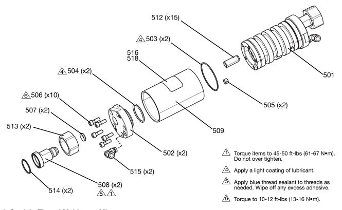
Fig. 6: Straight Thread Multi-pass Mixer
