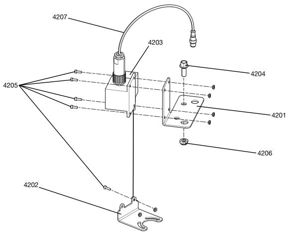
Fig. 43: Continuous Level Sensor 25A101
