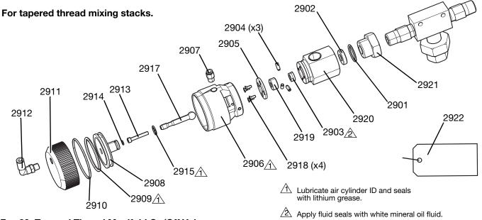
Fig. 30: Tapered Thread Manifold On/Off Valves
