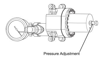
On all of the regulator models, the input line is connected to the port marked IN and the output line is connected to the port marked OUT. All models include a ball valve for bleeding the line, if needed.
