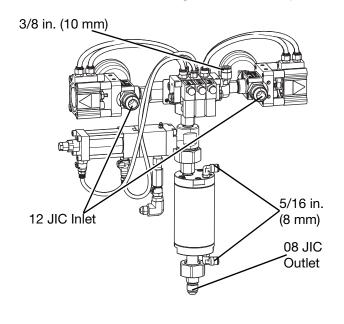
The 25A876 Mixer comes from the factory with 15 mixer cartridges, making a total of 30 mixing elements. It is possible to reduce the pressure drop through the mixer by using fewer mixing elements.
