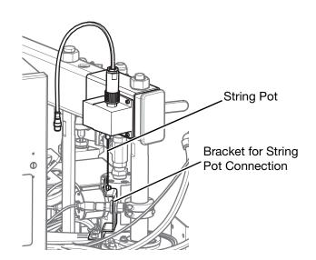
Attach the string pots (4102) to the string connection brackets located on the electronic enclosure brace. Use the screws (4103) included in the continuous level sensor kit to attach the string to the bracket on each side.
