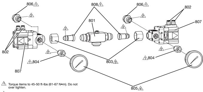
Apply blue thread sealant to threads as needed.
