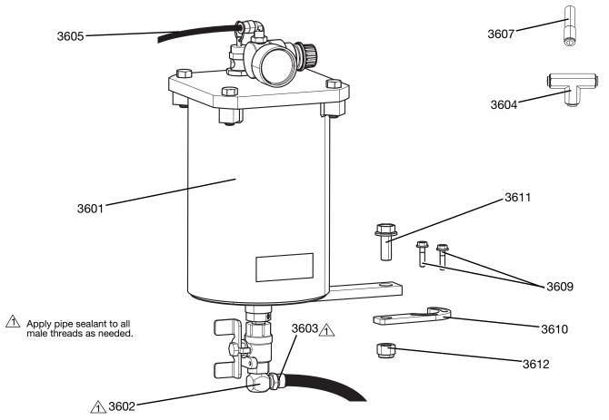
Fig. 37: Colorant Tank 25A104
