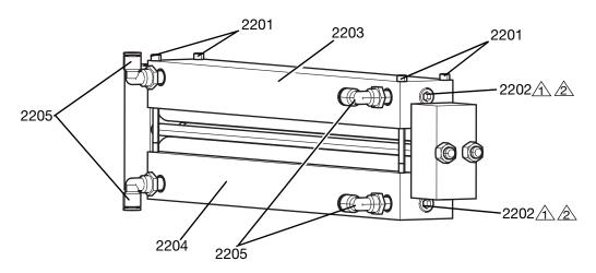
Apply a light coating of anti-seize lubricant to all male threads as needed.
