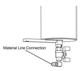
**NOTE:** The connection for the material line depends on if you are using a color flow meter or not. See **Color Flow Meter Kits** and **Color Injector Kits** on page **22** to complete installation.
