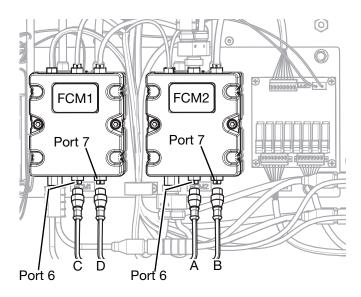
5. Insert the custom software blue token included in the kit into FCM2. This is required to run the machine in small shot mode.
