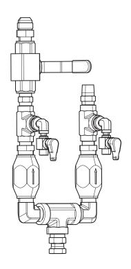
Remove the material outlet ball valve and adapter fitting from the machine where you are installing the dual press kit.
