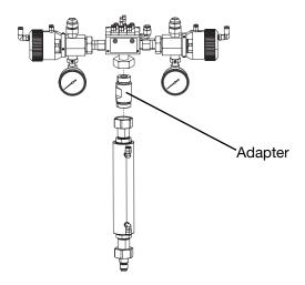
Connect the 1-1/14 in. end of the adapter to the tapered thread stack's manifold and the 1-3/8 in. end of the adapter to the mixer (25C003 shown). Tighten the connections at both ends until secure.
