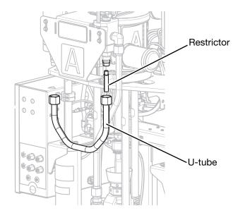
**NOTE:** If there is material in the tube, clean out enough of it to allow the restrictor to be completely inserted into the tube.
