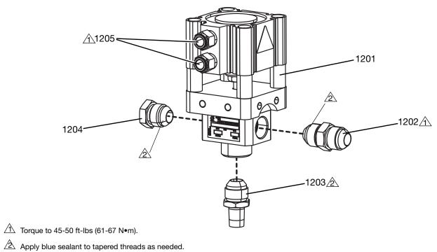
Fig. 13: Straight Thread Shut-off Valve
