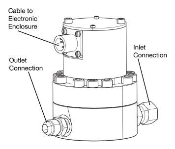
Connect the other end of the cable to the electronic enclosure at one of the Color F/M connections. See page 9 for a diagram of the electronic enclosure's connections. **NOTE:** Always use Color F/M 1 if you are only using one press. Color F/M 2 can be used for the second connection in a dual press configuration, or if two injectors are used on a single press.
