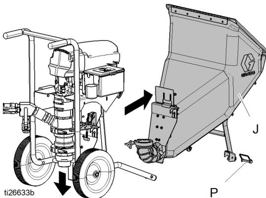
**NOTE:** If the hopper elbow needs to be thoroughly cleaned, rotate the second knob (K) to loosen the clamp between the elbow and the hopper. Remove and clean the elbow.
