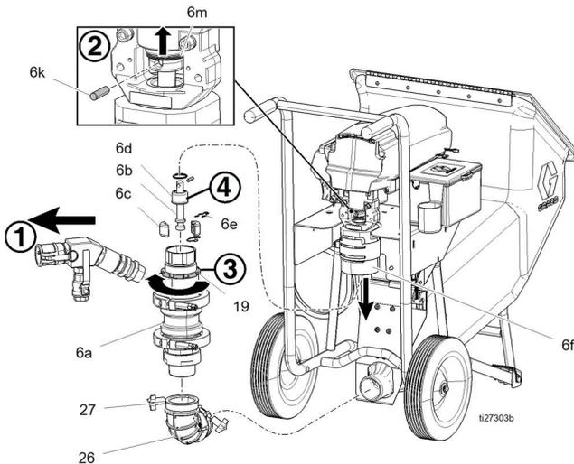
**NOTE:** When reinstalling the pump lower, the jam nut (19) should be threaded on the pump lower until it bottoms out. The pump lower should be threaded completely into the motor adapter (6f) and backed off to the correct orientation position shown below. Once in position, unthread the pump two additional turns and secure the jam nut.
