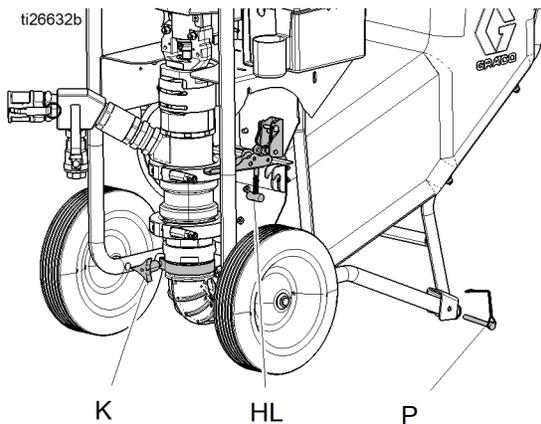
3. Remove the locking pin and pull down the hopper latch (HL) on the hopper plate.
