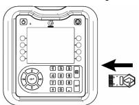
**NOTE (PC-8e systems only):** Remove the blue key token 24X626 to install the update. Re-install the blue key token after the software update.
