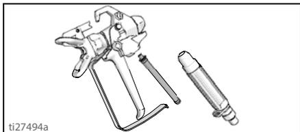
2. Remove spray tip and tip guard and clean with water or flushing fluid and a brush.
