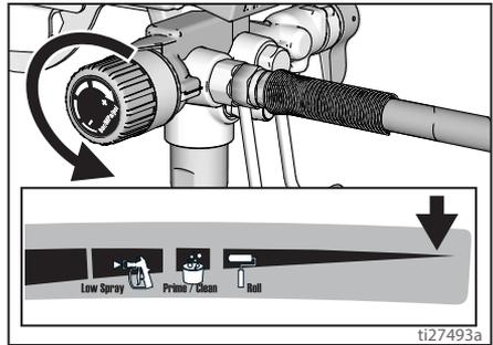
4. Put drain tube into a waste pail and place Prime/Spray valve in **PRIME** position (drain) to relieve pressure.
