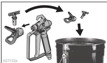
3. Wipe paint off outside of gun using a soft cloth moistened with water or flushing fluid.
