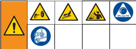
This equipment stays pressurized until pressure is manually relieved. To help prevent serious injury from pressurized fluid, such as skin injection or splashed fluid, follow the **Pressure Relief Procedure** whenever sprayer is stopped and before sprayer is cleaned or checked, and before equipment is serviced.
