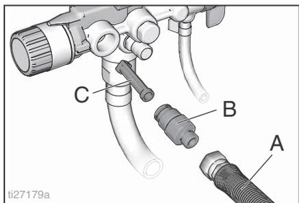
5. Check InstaClean Fluid Filter (C) for debris. If needed, clean filter with water or flushing fluid and a soft brush.
