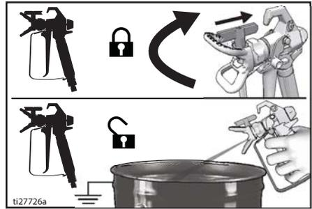
**NOTE:** If spray tip is difficult to rotate when turning to the unclog position perform, **Pressure Relief Procedure**, page 11, then turn Prime/Spray valve to spray position and repeat step 1.
