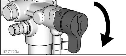
4. Turn ON/OFF switch to **ON** position.
