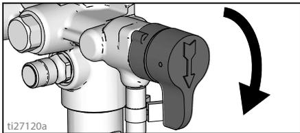
20. Turn ON/OFF switch to OFF position.
