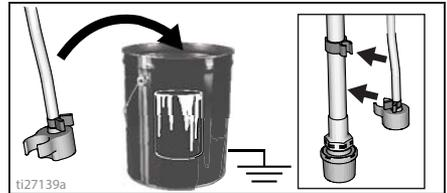
**NOTE:** When motor stops, sprayer is ready to paint. If motor continues to run, sprayer is not properly primed. Repeat **Fill Pump** and **Fill Gun and Hose**.
