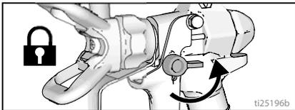
5. Remove tip guard. Be careful tip seal may fall out when tip guard is removed.
