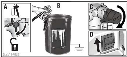
13. While continuing to trigger gun, quickly move gun to redirect spray into waste pail. Continue triggering gun into waste pail until flushing fluid dispensed from gun is relatively clear.
