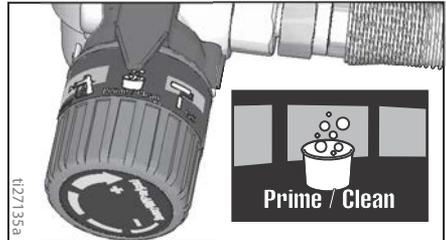
8. Turn Prime/Spray valve down to PRIME position.
