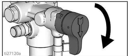
5. Hold the gun firmly to a pail. Point gun into pail. Disengage the trigger lock and trigger the gun to relieve pressure.
