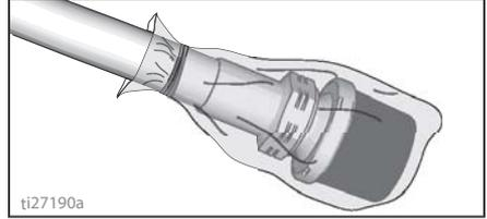
11. Secure a plastic bag around suction and drain tube to catch any drips.
