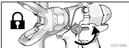
16. Turn Prime/Spray valve down to PRIME position.
