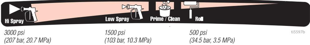
To select function, align symbol on pressure control knob with setting indicator on sprayer.
