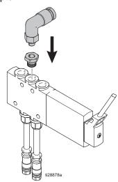
**Step 2 (Metric Only):** Install 90° fitting (129174) directly into the solenoid valve. Adapter (17L982) is not needed and can be thrown away.
