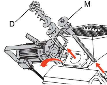
**NOTE:** Only use the clean-out shaft (M) if material cannot be cleaned using normal flushing means. Excessive use of the clean-out shaft can cause premature wear to the system.
