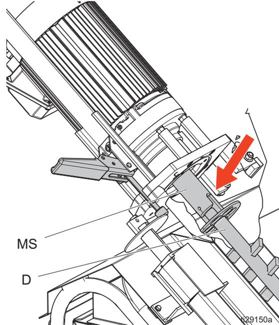
4. Swing the motor completely shut and lock it in place with the motor latch (K).
