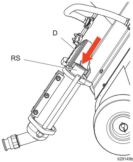
2. Slowly swing the motor assembly toward its closed position, stopping shortly before the motor shaft adapter (MS) and drive/mix shaft (D) touch.
