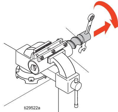
3. Replace the worn rotor (27) or stator (28) with a new part, then screw the rotor (27) clockwise back into the stator (28).
