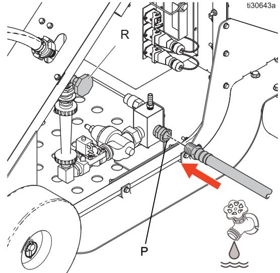
**NOTE:** The water feed must be able to supply water pressure of 30 psi or greater at the desired flow rate, or else the pump will not operate in the forward direction. A pressure switch that controls the pump forward direction operation activates at 30 psi to allow forward operation. If water pressure is below 30 psi and the pump must be operated in the forward direction, the pressure switch can be bypassed by connecting the water pressure bypass plug.
