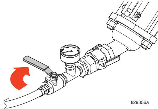
7. Observe the pressure setting on the pressure gauge.
