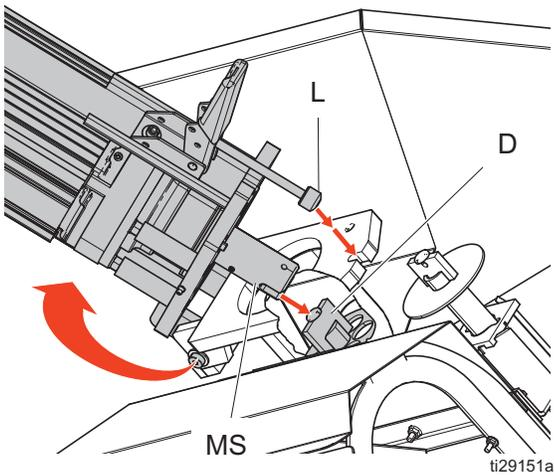
3. Make sure the motor shaft adapter (MS) and drive/mix shaft (D) are aligned so the drive shaft flat slides into the motor shaft adapter slot. If they do not align, rotate them into position.
