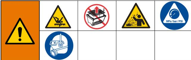
To help prevent injury from moving parts, do not operate with the grate (J) removed.
