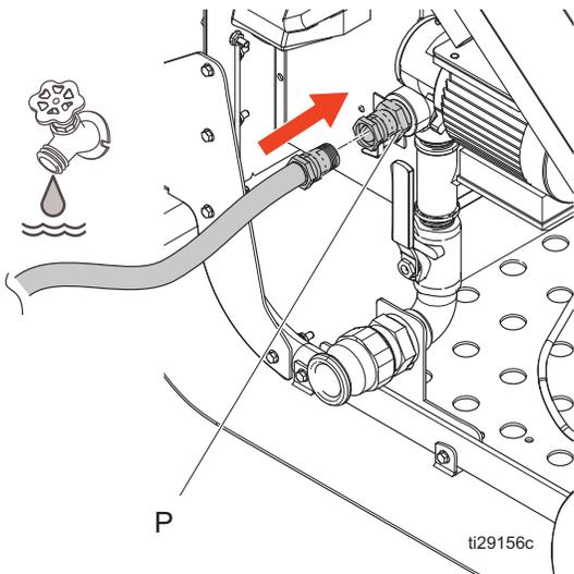
**NOTE:** The water feed must be able to supply water pressure of 30 psi or greater, or else the pump will not operate in the forward direction. A pressure switch that controls the pump forward direction operation activates at 30 psi to allow forward operation. If water pressure is below 30 psi and the pump must be operated in the forward direction, the pressure switch can be bypassed by connecting the water pressure bypass plug.
