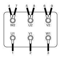
b. **For 230V Motors:** Move the 7, 8, and 9 wires as shown. Bridge W2, U2, and V2 as shown.
