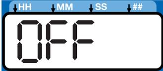
2. Press the UP or DOWN ARROW to change OFF to ON on the display to change the alarm output to be on steady.
