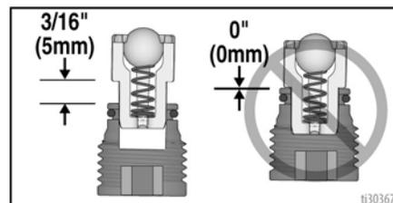
8. Check ball should move freely against the spring in the retainer.
