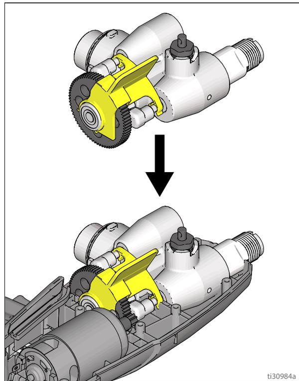
7. On a brushless sprayer, use a wrench to hold the pump bearing. Install the static dissipation wire screw. See assembly drawings for torques.
