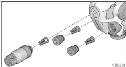
3. To remove the three outlet valves, remove two pump plugs (4b) and front valve (25). Use 8mm (5/16") Allen wrench to remove pump plugs. On the Ultra MAX, Ultimate MX, and TC PRO PLUS (Brushless) sprayers use the removal/installation tool provided to remove the front valve.
