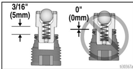
6. Check ball should move freely against the spring in the retainer.
