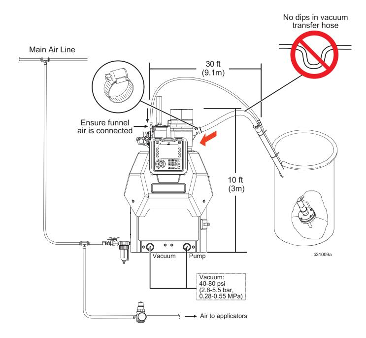
**NOTE:** See the system manual for required system installation settings.
