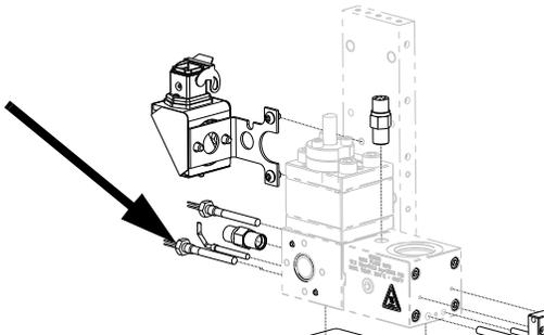
6. Remove the heaters and sensor from the block.
