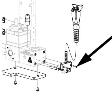
4. Remove two M6 screws to remove the kit from the pump block.
