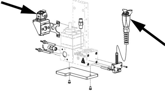
3. Remove two M3 screws to remove the kit from the inlet block.
