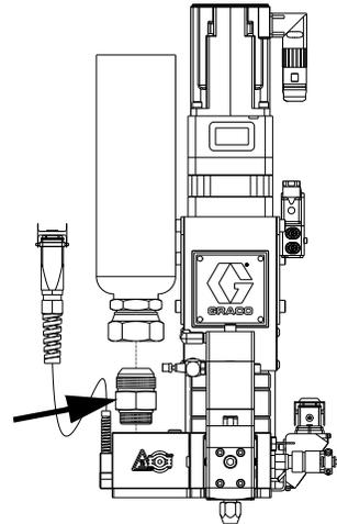
**FIG. 8: Inlet Fitting**
