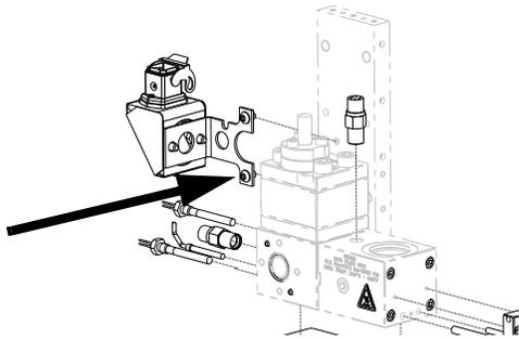
5. Remove the two M8 heater nuts and M6 sensor nut.
