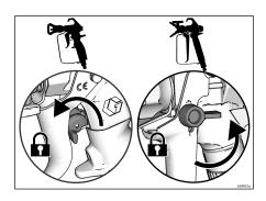
3. Turn pressure control to the lowest setting. Disengage the trigger lock.
