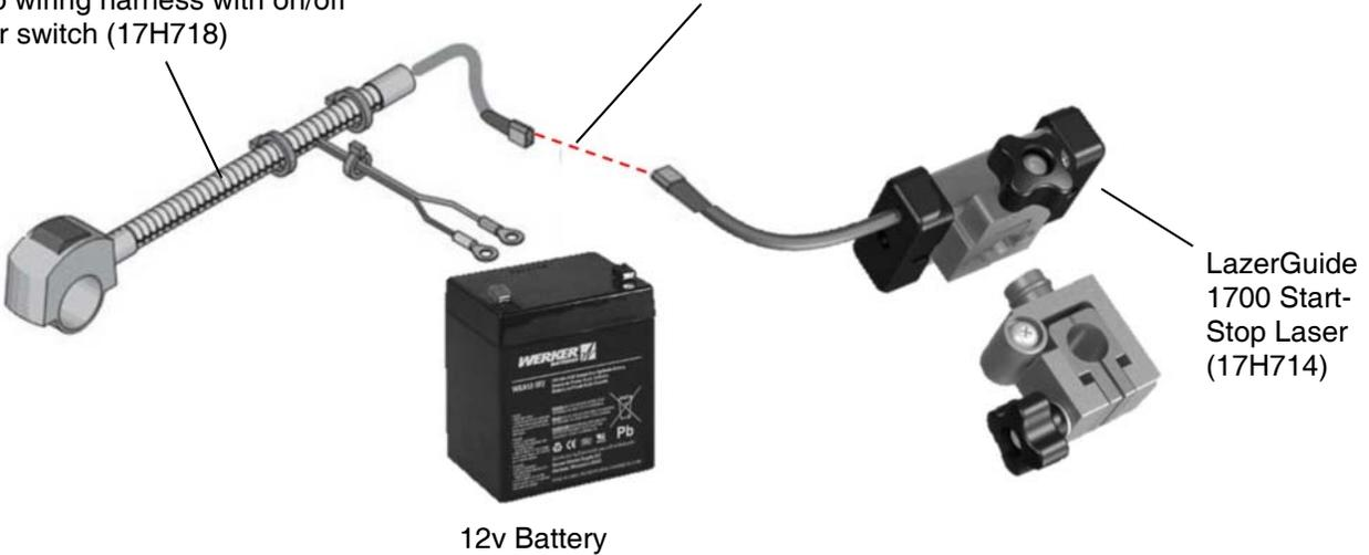
Insert provided Graco "Y" cable adapter (17T537) to the wiring harness as shown. Then connect both the LazerGuide 2000 and LazerGuide 1700 to either one of the two connectors.
