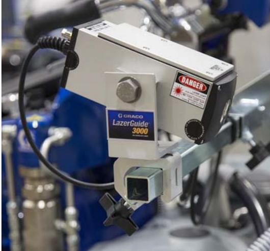
2. Turn laser ON by turning on the sprayer.
