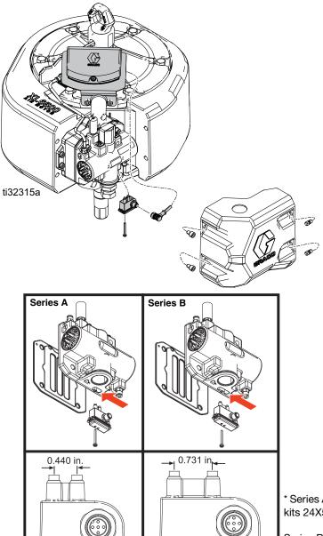
\* Series A air valves are needed for kits 24X550 and 24X552.
