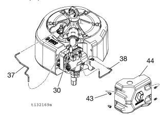
4. Remove six screws (27) and remove the manifold and valve (30) and two gaskets (24). Inspect foam for damage.
