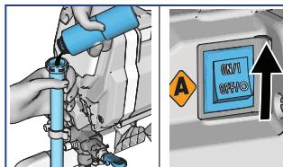
**3** While holding the Suction Tube above the sprayer, pour approximately 2 ounces (1/4 cup) of Pump Armor into the Suction Tube and turn Power Switch ON.
