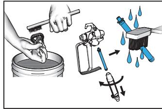
**7** Clean Spray Tip, Spray Tip Guard and inlet screen with brush. Remove gun filter and clean. Reassemble gun filter, Spray Tip and Spray Tip guard.
