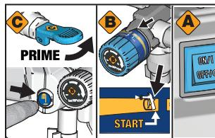
**3** Lift the Prime/Spray Valve to the PRIME position. Press the PushPrime button\* twice to loosen inlet valve ball. Turn Pressure Control Knob to START position. Turn Power Switch ON.
