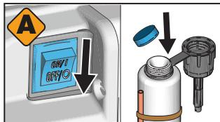
**4** When Pump Armor is flushed through the sprayer, turn Power Switch OFF. Replace and tighten child-proof cap for storage.
