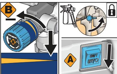
**6** Turn Pressure Control Knob to lowest setting and release trigger. Engage Trigger Lock. Lift Prime/Spray Valve to PRIME and turn Power Switch OFF.
