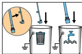
**2** Separate Drain Tube (smaller) from Suction Tube (larger). Place Drain Tube in a waste pail. Submerge Suction Tube into pail filled with water for water-based material, or mineral spirits if spraying oil-based material.
