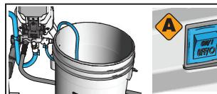
**4** Allow fluid to flow up the Suction Tube and out of Drain Tube for 30-60 seconds. Turn Power Switch OFF.
