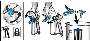
**2** Engage Trigger Lock. Remove Spray Tip Guard assembly from gun and place in waste pail.
