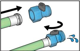
**3** Screw Power Flush Valve (included with sprayer) to a garden hose. Turn on water. Open Power Flush Valve. Rinse paint off Suction and Drain Tubes, inlet screen and Spray Tip and Spray Tip Guard. Close Power Flush Valve.
