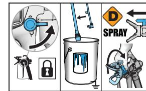
**7** When paint comes out of gun, release trigger. Engage Trigger Lock. Transfer Drain Tube to paint pail and attach to Suction Tube. Rotate Spray Tip back to SPRAY position and ensure Spray Tip Guard is tight.
