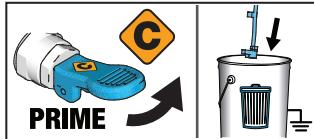
**2** Lift Prime/Spray Valve to PRIME. Place Drain Tube in waste pail. Turn Pressure Control Knob to START position.
