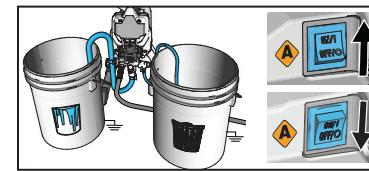
**5** Submerge Suction Tube into paint. Turn Power Switch ON and watch for paint to come out of the Drain Tube. Turn Power Switch OFF.
