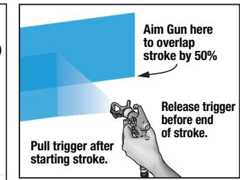
**2** Increase Pressure Control Knob if needed until spray is even and without gaps at edges.
