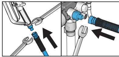
**1** If needed, connect hose to gun. Remove red cap, then connect hose to sprayer. Tighten securely.
