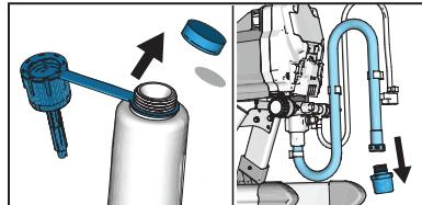
**1** Remove Pump Armor bottle cap and foil seal. If needed, unscrew inlet screen from Suction Tube.
