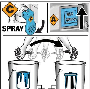
**5** To save paint in hose, disengage Trigger Lock and trigger gun into paint pail, lower Prime/Spray Valve to SPRAY and turn Power Switch ON. When water comes out of gun, keep gun triggered and aim into waste pail. Continue to flush until water runs clear.
