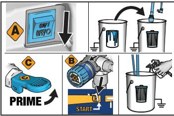
**1** Turn Power Switch OFF. Place Suction and Drain Tubes in waste pail. Lift Prime/Spray Valve to PRIME. Turn Pressure Control Knob to START position. Trigger gun into a waste pail.
