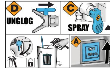
**6** Rotate Spray Tip to UNCLOG Position. Disengage Trigger Lock. Point gun into waste pail, pull and hold trigger. Lower Prime/Spray Valve to SPRAY position and turn Power Switch ON.
