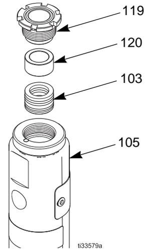
**Fig. 8 Top packing seal assembly**
