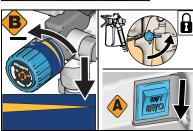
6 Turn Pressure Control Knob to lowest setting and release trigger. Engage Trigger Lock. Move Prime/Spray Valve to PRIME and turn Power Switch OFF.
