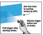
Increase Pressure Control Knob if needed until spray is even and without gaps at edges.
