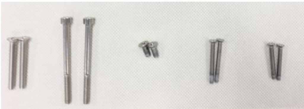
L-R: top cover (2), nozzle plate (2), mounting plate (2), heater block (2), spacer (2)
