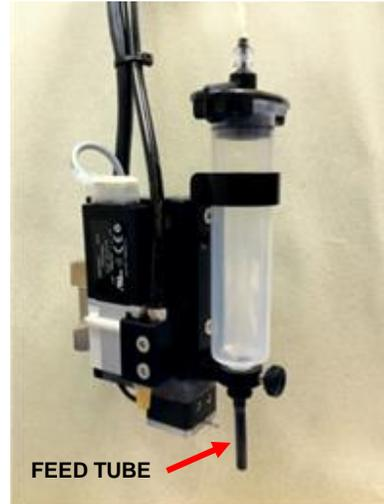
3. Slip the feed tube onto the barb end of the nozzle plate.
