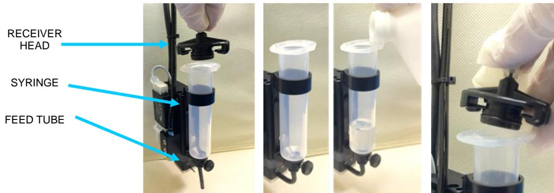
6. Fill the syringe with about 3 cc of mild solvent compatible with your fluid material.
