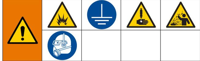
To avoid fire and explosion, always ground equipment and waste container. To avoid static sparking and injury from splashing, always flush at the lowest possible pressure.
