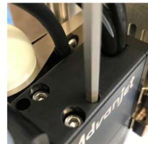
9. Before installing the fluid syringe, CLOSE the jet.
