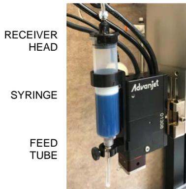
Figure 4-3: Disassemble and Remove Syringe
