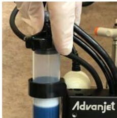
4. Attach a new feed tube to the luer (metal luer shown; selection of feed tube material depends on the dispensing fluid).
