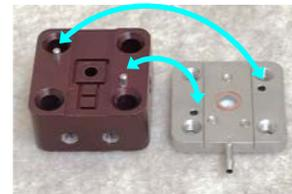
7. Use the pins to align the nozzle plate on the heater block. The nozzle plate O-ring faces up, and the fluid barb faces the fluid syringe.
