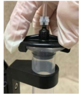
Figure 4-3: Replace Receiver Head
