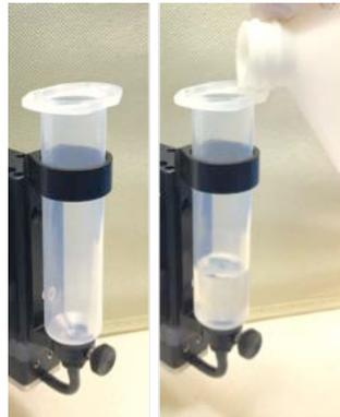
Figure 4-3: Install an Empty Syringe and Fill With Solvent
