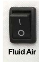
2. Turn the **Fluid** (melter) heat OFF:
