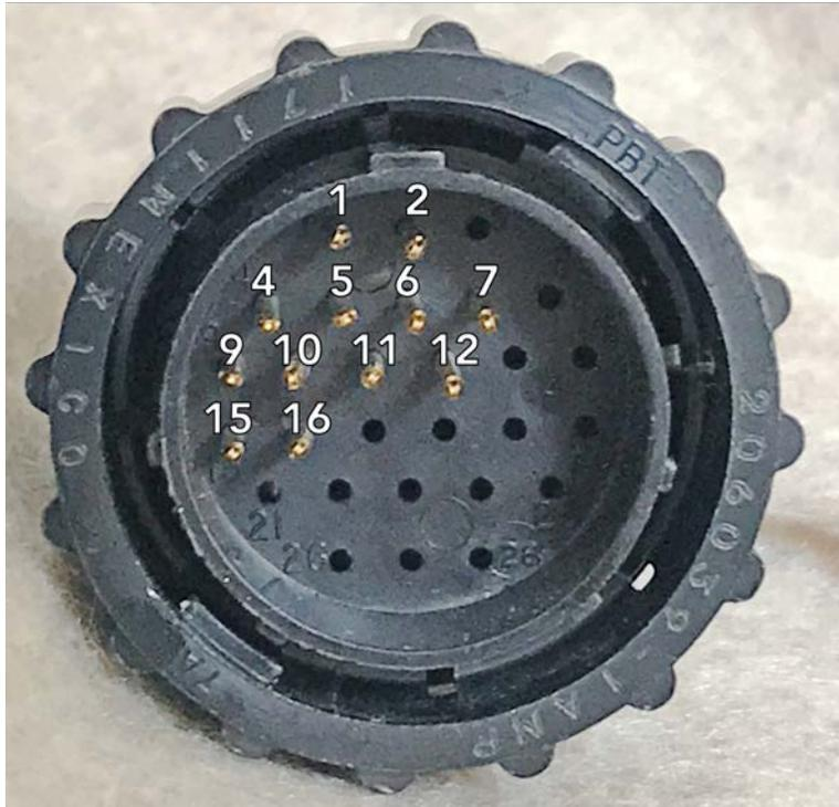
Figure 2-4: 28-Pin Jet Cable
