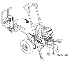
5. Look through side vent holes and ensure drive belt is in motor pulley.
