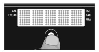
The sprayer model briefly displays (e.g. 5900), SERIAL NUMBER scrolls past and then serial number (e.g. 00001) displays.
