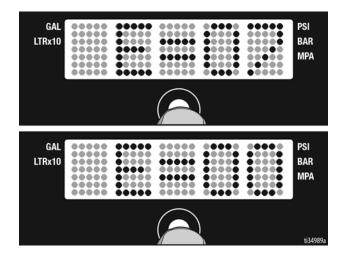
Short press **DISPLAY** button. **W-DOG** scrolls past then **OFF** displays if watchdog switch is OFF. **ON** displays if Watchdog switch is ON.
