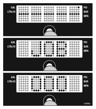
**NOTE: JOB** scrolls past, then the number of gallons sprayed above 1000 psi (70 bar, 7 MPa) displays.
