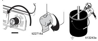
2. Turn power ON. Pressure display appears. Dashes will not appear unless pressure is less than 200 psi (14 bar, 1,4 MPa).
