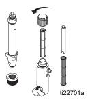
Fill throat packing nut with TSL to prevent premature packing wear. Do this each time you spray.
