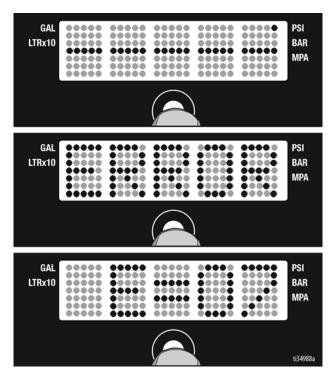
Press and hold **DISPLAY** button to clear error code to zero.
