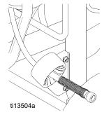
2. Lift and turn pivot lock 90 to unlock hose reel. Pull on hose to remove it from hose reel.
