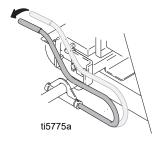
3. Remove engine; tilt and slide back.
