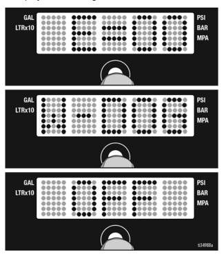
Short press **DISPLAY** button to move to Watch Dog sensitivity menu. Press and hold **DISPLAY** button Watch Dog can be set to low, medium, or high sensitivity. Release **DISPLAY** button when desired sensitivity setting is displayed.
