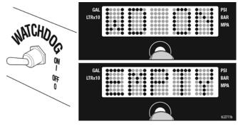
Turn WatchDog switch OFF. Add material or reprime sprayer. Turn pump switch OFF and ON to reset WatchDog protection system. Turn WatchDog switch back ON to continue to monitor material level.
