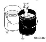
Turn prime valve down to DRAIN position. Turn pressure control counterclockwise to lowest pressure.
