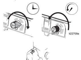
7. Disengage spray gun trigger lock.
