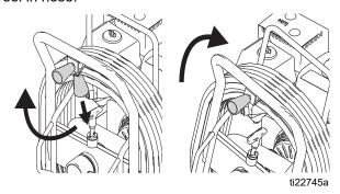
**NOTE:** The QuikReel can be locked into two positions: Usage (A) and Storage (B).
