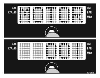
Short press DISPLAY button. LAST ERROR CODE scrolls by and last error code is displayed; e.g. E=07. See sprayer Repair manual for additional information.
