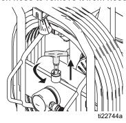
3. Pull reel handle down and out. Turn clockwise to reel in hose.
