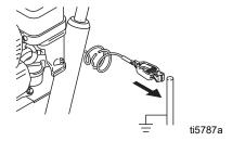
**To ground sprayer:** Attach sprayer grounding clamp to earth ground.
