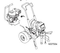
4. Install motor; drop in and push forward.
