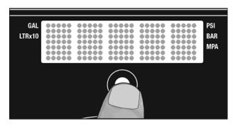
Turn pressure to lowest setting. Trigger gun to relieve pressure. Turn prime valve down to DRAIN position.
