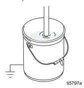
11. Trigger gun again into flushing fluid pail until material appears.
