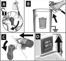
15. While continuing to trigger gun, quickly move gun to redirect spray into waste pail. Continue triggering gun into waste pail until flushing fluid dispensed from gun is relatively clear.
