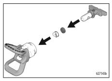
Spray Tip must be pushed all the way into the Spray Tip Guard. Rotate Spray Tip while pushing down.
