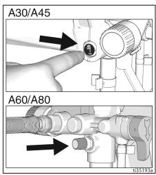
7. Align setting indicator with the **START** setting on the pressure control knob.
