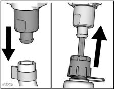
4. Squeeze Pump Armor bottle until Pump Armor flows into the Drain Tube.
