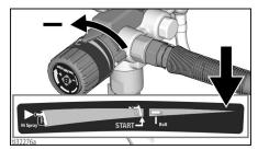
Put Drain Tube into a waste pail and move Prime/Spray Valve to PRIME position to relieve pressure.
