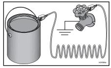
To maintain ground continuity when sprayer is flushed or pressure is relieved: hold metal part of gun firmly to the side of a grounded metal pail, then trigger the gun.
