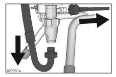
5. Slide pump out of the drive housing.
