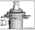
Move pump displacement rod up or down until it slides into the connecting rod when the pump is slid into the drive housing.
