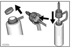
3. Remove sprayer Suction Tube. Insert tool into the inlet and push up firmly until it stops.
