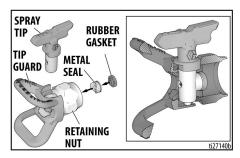
a. Use Spray Tip to align gasket and seal in the Spray Tip Guard.
