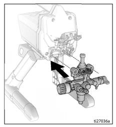
a. Move pump rod up or down until cap is level with the opening in the yoke.
