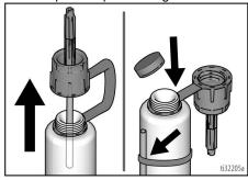
6. Reinstall the sprayer Suction Tube. Ensure that the tube is snug on the inlet and the clamp is engaged.
