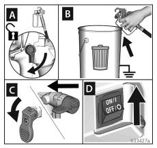
3. Trigger gun into waste pail until only paint comes out of the gun.
