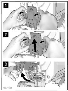
Slide pump assembly off the mounting pins.
