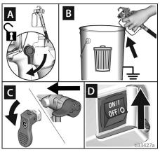
e. Continue to hold gun trigger until you see paint diluted with flushing fluid starting to come out of gun.
