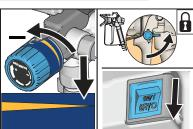
Control Knob to lowest setting and release trigger. Engage Trigger Lock. Turn the Prime/Spray Valve to PRIME and turn Power Switch OFF.
