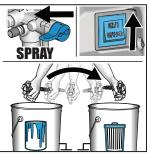
5 To save paint in hose, disengage Trigger Lock and trigger gun into paint pail, turn Prime/Spray Valve to SPRAY and turn Power Switch ON. When water comes out of gun, keep gun triggered and aim into waste pail. Continue to flush until water runs clear.
