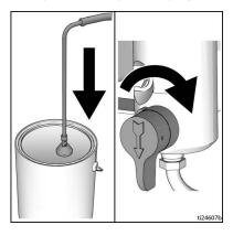
Hold a metal part of the spray gun firmly to a grounded metal pail. Point spray gun into pail. Disengage the trigger lock and trigger the spray gun to relieve pressure.
