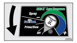
Put drain tube in a pail and turn prime valve down to relieve pressure. Leave prime valve in the down (drain) position until you are ready to spray again.
