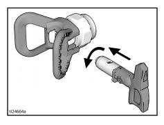
4. Screw assembly onto gun. Tighten.
