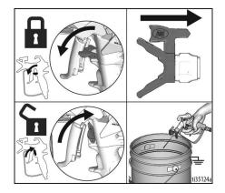
Engage trigger lock. Return Spray Tip to original position. Disengage trigger lock and continue spraying.
