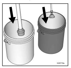
5. To flush drain tube and pump turn prime valve down.
