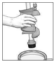
Place fluid intake in flushing fluid. Use water for water base paint and mineral spirits for oil-based paint. Place drain tube in waste pail.
