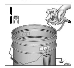
Move gun to paint pail and trigger for 20 seconds. Release trigger and allow sprayer to build pressure. Engage trigger lock.
