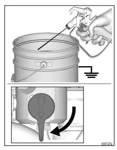
Turn pressure control to Fast Flush operate until the pump runs steady and flushing fluid appears in the waste pail.
