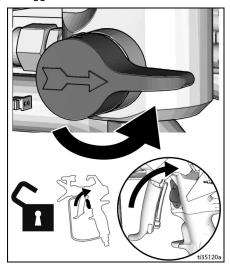
7. Hold gun against grounded metal waste pail. Trigger gun until paint appears.
