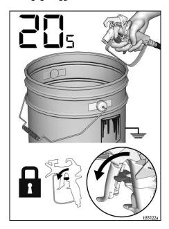
Turn pressure control knob to OFF and turn ON/OFF switch to OFF position. Disconnect power to sprayer.
