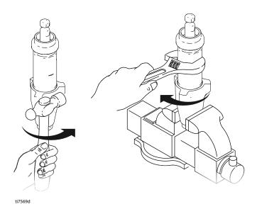
13. Torque packing nut (202) as follows:
