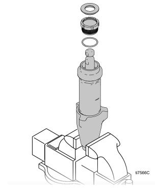
2. Unscrew intake valve from cylinder.
