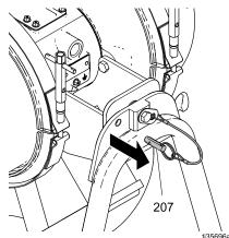
**NOTE:** After draining, rotate the pump to positions which will aid disassembly.
