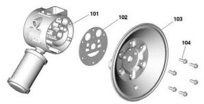
7. Remove the air cover gaskets (102). Always replace the gaskets with new ones.
