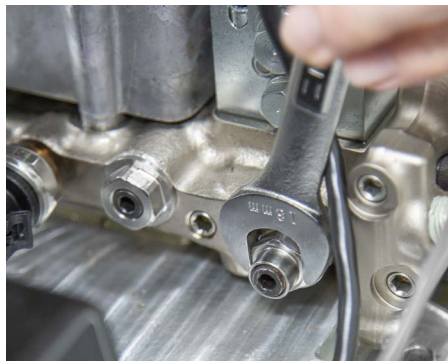
1,500 psi relief valve shown
