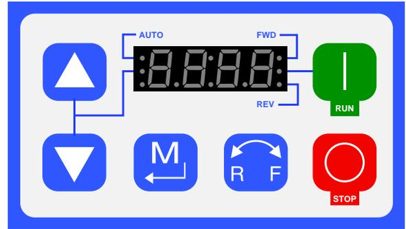
Figure 7 Panel de control del VFD
