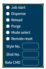
The input signals display shows the current signal status from customer inputs.
