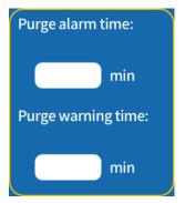
Set the purge request time. When the equipment doesn't dispense, the PSM control box will start the countdown for the time chosen by the operator. When time is up, the system will send out the purge alarm signal and show 'purge request' in the information bar.
