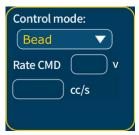
In Bead mode with custom setting, 'Rate CMD' will be shown as voltage value and target flow rate will be shown. The flow rate will change based on rate command.
