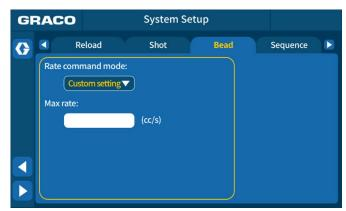
Fig. 22 Bead Setup Screen (Custom setting)
