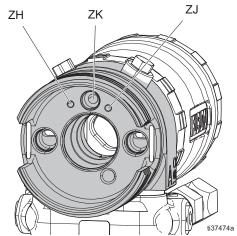
Fig. 3 Fluid Housing Passages
