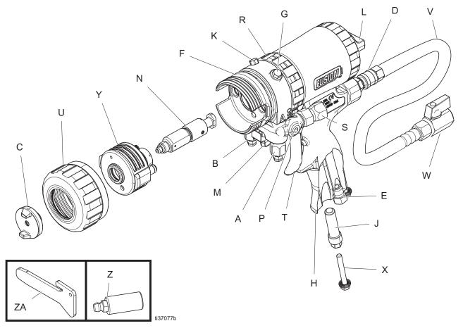
Fig. 1 Component Identification
