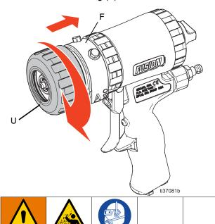
To prevent damage to the fluid o-ring or injury from splashing chemical, verify that the fluid cartridge (Y) is fully engaged into the fluid housing (F), and the front retaining ring (U) is tight.
