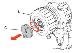
Remove the PC fluid cartridge (Y) by pulling forward or inserting a screwdriver into the pry slots. Sealing surfaces and opposing checks will cause resistance.
