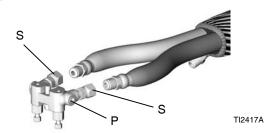
Apply thread sealant to plugs (12c), elbows (50), and male threads of fluid inlet swivels (S). Install elbows (50) in optional fluid inlets (P), facing down. Install swivels (S) in elbows. Be sure to install A swivel (smaller) in A side. Install included plugs where swivels were located. Torque all parts to 235-245 in-lb (26.6-27.7 N•m).
