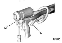
3. Unscrew cylinder cap (5). Hold piston stop (28) with wrench and unscrew from safety lock (4). Inspect spring (30) and o-rings (14, 24).
