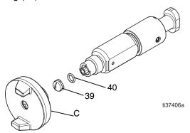
**NOTE:** If tip is stuck, pry off with small screwdriver or pull off with pliers. Tip is hardened to resist damage.
