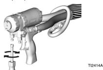
12. Disengage the piston safety lock (L). See **Piston Safety Lock**, page 20.
