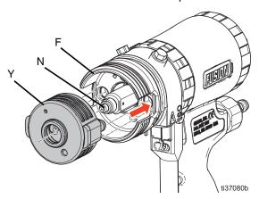
c. Fully engage the fluid cartridge (Y) into the fluid housing (F) until the back face of the cartridge is flush with the fluid housing.
