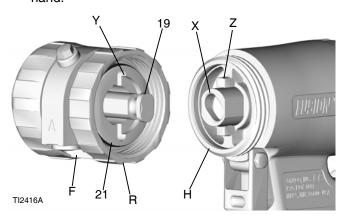
Turn fluid housing 1/8 turn clockwise to engage slots (Y) and tabs (Z). Push on front end to ensure it is properly seated. Continue screwing lock ring (R) onto handle (H) very securely. When properly assembled, lock ring is snug against handle.
