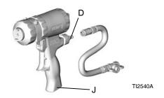
Reattach the fluid manifold. Reconnect air. Return gun to service.
