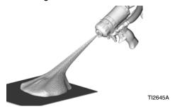
14. Apply layer of lubricant over front of gun and lock ring (R), or use gun cover to prevent overspray buildup and aid disassembly. See page **Lubricant for Gun Rebuild**, page 43, to order lubricant and gun cover.
