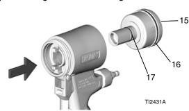
7. Liberally lubricate piston o-rings. Reinstall piston. Shaft is keyed for proper assembly. Push firmly to seat piston.
