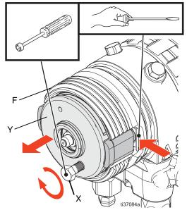
**NOTE:** If excessive force is required to remove the PC fluid cartridge, use the provided nut driver and jack screw (X) to lift the cartridge out of the fluid housing (F).
