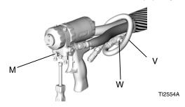
5. Connect the air line quick coupler (D). Turn on air. Open air valve (W). Air should flow from the mix chamber nozzle (N).
