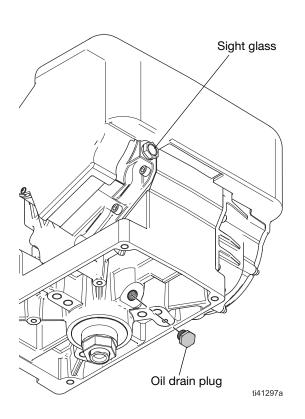
FIG. 15 Oil drain plug
