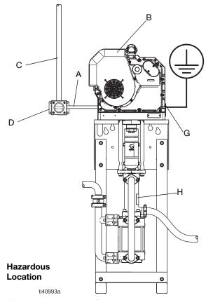
FIG. 3 Typical Installation (no communication module)
