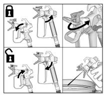
Engage trigger lock. Rotate spray tip back to spray position. Disengage trigger lock and continue spraying.
