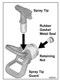
a. Use spray tip to align gasket and seal in the tip guard.
