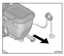
b. While holding the drain tube retainer with drain tube parallel to the top of a waste pail, twist retainer over the lip of the pail. Drain tube should now be inside the waste pail.
