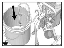
c. Submerge suction tube in a grounded pail partially filled with water or flushing fluid. When flushing with oil-based or flammable materials, follow **Grounding Instructions**, page 10.
