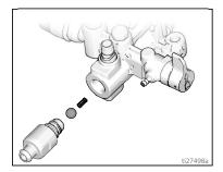
3. Clean any debris and dried paint from the cavity and replace the ball and spring. Tighten inlet valve to pump using integrated tool on the frame.
