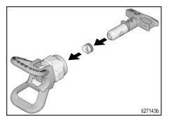
b. Spray tip must be pushed all the way into the tip guard. Turn spray tip to push down.
