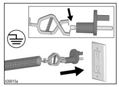
Fluid hoses: Use only electrically conductive hoses with a maximum of 300 ft. (91 m) combined hose length to ensure grounding continuity.
