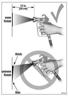
Flex wrist to keep gun pointed straight. Fanning gun to direct spray at angle causes uneven finish.
