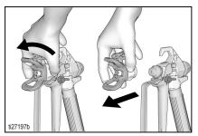
Remove suction tube and drain tube from paint, wipe excess paint off outside.
