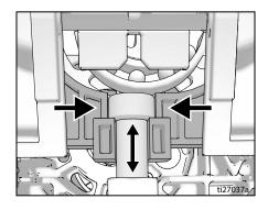
Swing easy access door pump door closed while pushing the entire door towards the inlet end of the pump.
