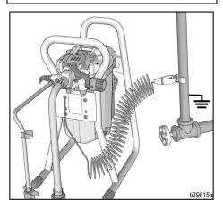
The sprayer is equipped with a grounding wire and clamp. The clamp must be connected to a true earth ground when spraying or flushing oil-based or flammable materials.
