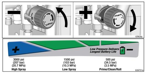
To select pressure, align symbol on pressure control knob with setting indicator on sprayer.
