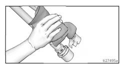
5. Separate drain tube (smaller) from suction tube (larger).
