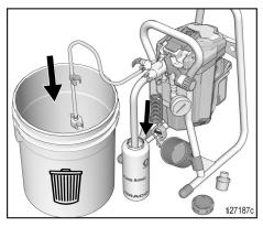
b. **For Hopper Models:** Pour Pump Armor into the hopper and place drain tube in waste pail.
