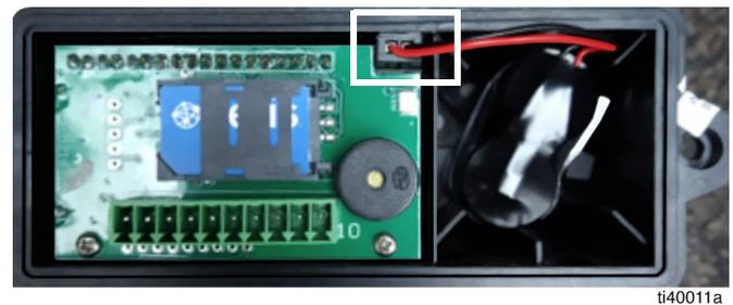
**FIG. 9 Disconnect Battery**
