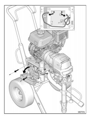
3. Loosen and remove four washers and four screws. Remove gear box assembly and pump.
