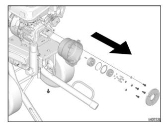
5. Loosen and remove two screws and two nuts. Remove engine.
