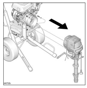
4. Remove clutch assembly and housing. Refer to **Pinion Assembly/Clutch Armature/Clamp** section in manual 3A6400.
