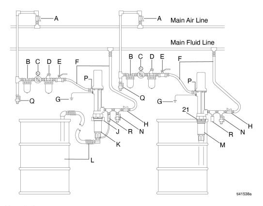
Fig. 1: Typical Installation
