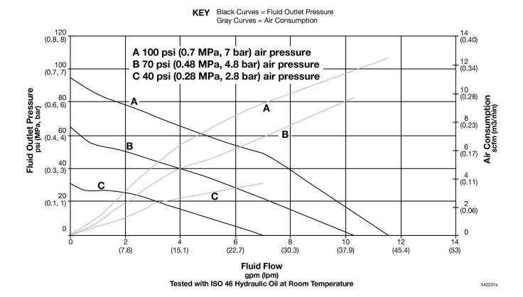
To find the fluid outlet pressure at a specific flow and operating air pressure:
