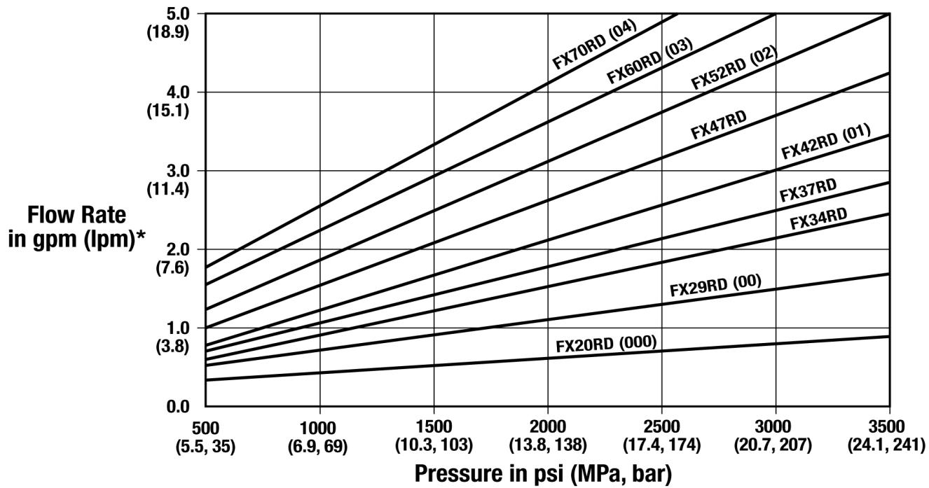
\* To calculate flow rate in lb/min., multiply gpm rate by 10.
