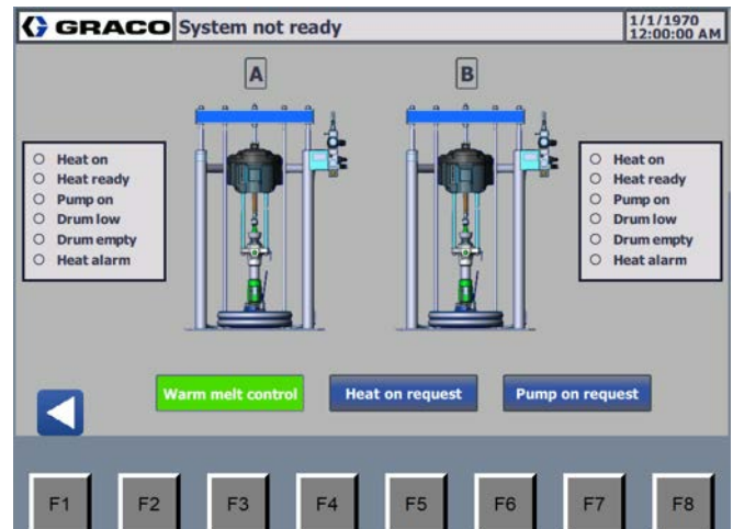
FIG. 29 Pump Heating Screen - Two Pumps
