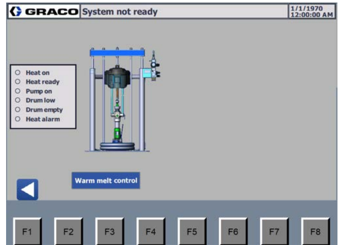
FIG. 28 Pump Heating Screen - One Pump
