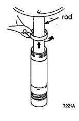
Unscrew the piston assembly tool from the cylinder. Clip the piston assembly tool with a diagonal cutter, and discard it.
