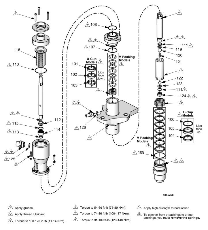
**NOTE:** Full disassembly shown. Disassemble only as far as needed for the parts being replaced.
