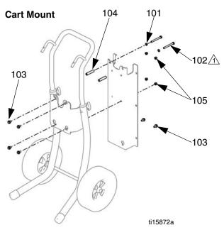
$\begin{tabular}{ll} $ \triangle \end{tabular} \label{eq:constraints} Apply red Loctite^\end{tabular}$  (included) approximately 0.25 in. on screw thread.
