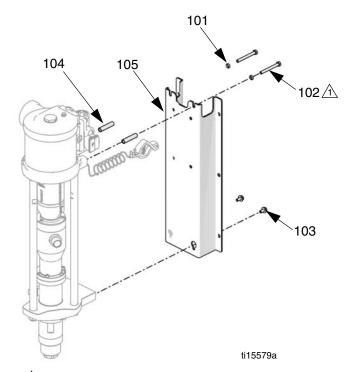
Apply red Loctite<sup>®</sup> (included) approximately 0.25 in. on screw thread.
