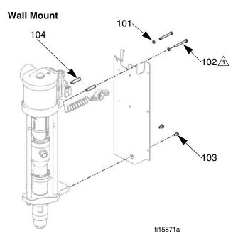
$\begin{tabular}{ll} $ \triangle \end{tabular} \label{eq:constraints} Apply red Loctite^{@} (included) approximately 0.25 in. on screw thread.$
