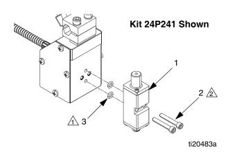
Apply high temperature lubricant 24T156 to o-rings.
