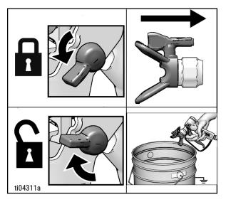
2. Engage Trigger Lock. Return Spray Tip to original position. Disengage Trigger Lock and continue spraying.
