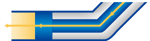
First-in-first-out (FIFO) fluid path
