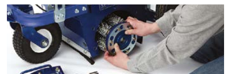
3. Remove drum assembly
