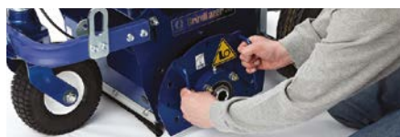
2. Remove bolts and door
