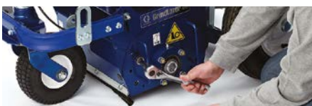
1. Loosen four bolts
